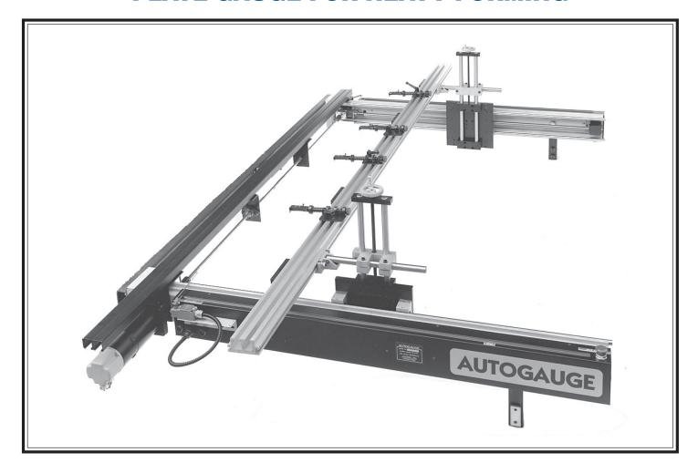
Programmable backgauging for pressbrakes has always offered impressive productivity savings for medium and short runs on light sheet metal. Now, the G48 for Pressbrakes brings those same savings when forming heavier materials.
